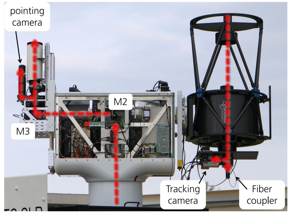
Basic principle of laser ranging. Emitted Transportable laser ranging station pulses are reflected by an object and returning photons are collected with a At the Institute of Technical Physics/ telescope.
