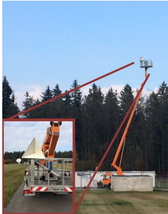
Figure 10. Photograph showing the setup for external calibration and frequency dependent error correction including antennas, feed systems and waveguides. A trihedral corner reflector in elevated position is used as well-known external radar target.
