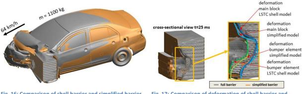
Fig. 16: Comparison of shell barrier and simplified barrier during the Euro NCAP load case (40% offset, 64 km/h impact speed)
