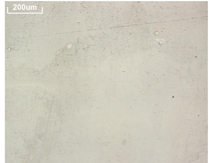
Glass surface corrosion
