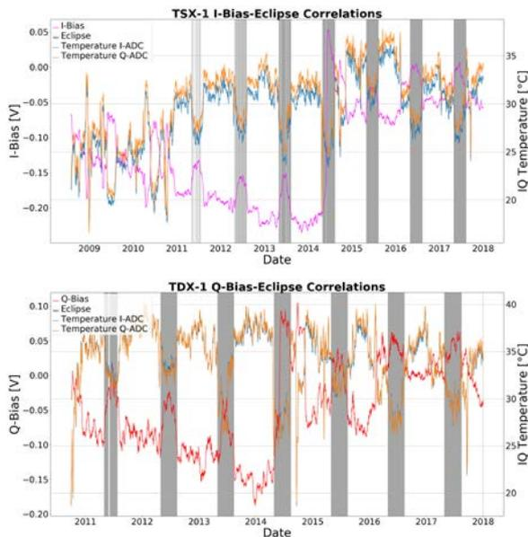
**Figure 3:** I/Q-Bias over mission duration. Upper plot: I-Bias TSX-1, lower plot: Q-Bias TDX-1
