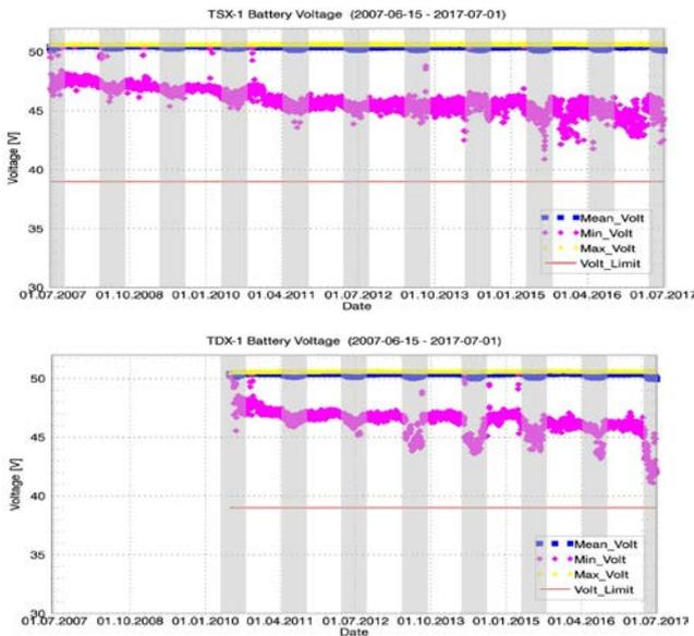
**Figure 1:** Battery voltage per day over mission duration and eclipse periods. Upper plot: TSX-1, lower plot: TDX-1
