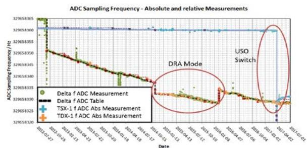
**Figure 2:** Relative and absolute ADC sampling frequency measurements of TSX-1 and TDX-1
