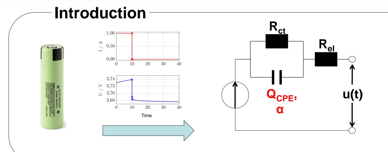
Equivalent circuit models are a common way to describe the electrochemical behavior of batteries and other electrochemical devices. Usually equivalent circuit parameters are obtained by fitting impedance spectra with a suitable model circuit. This work explores a method to fit fractional order equivalent circuits from time-domain relaxation measurements after current excitation of a battery.
