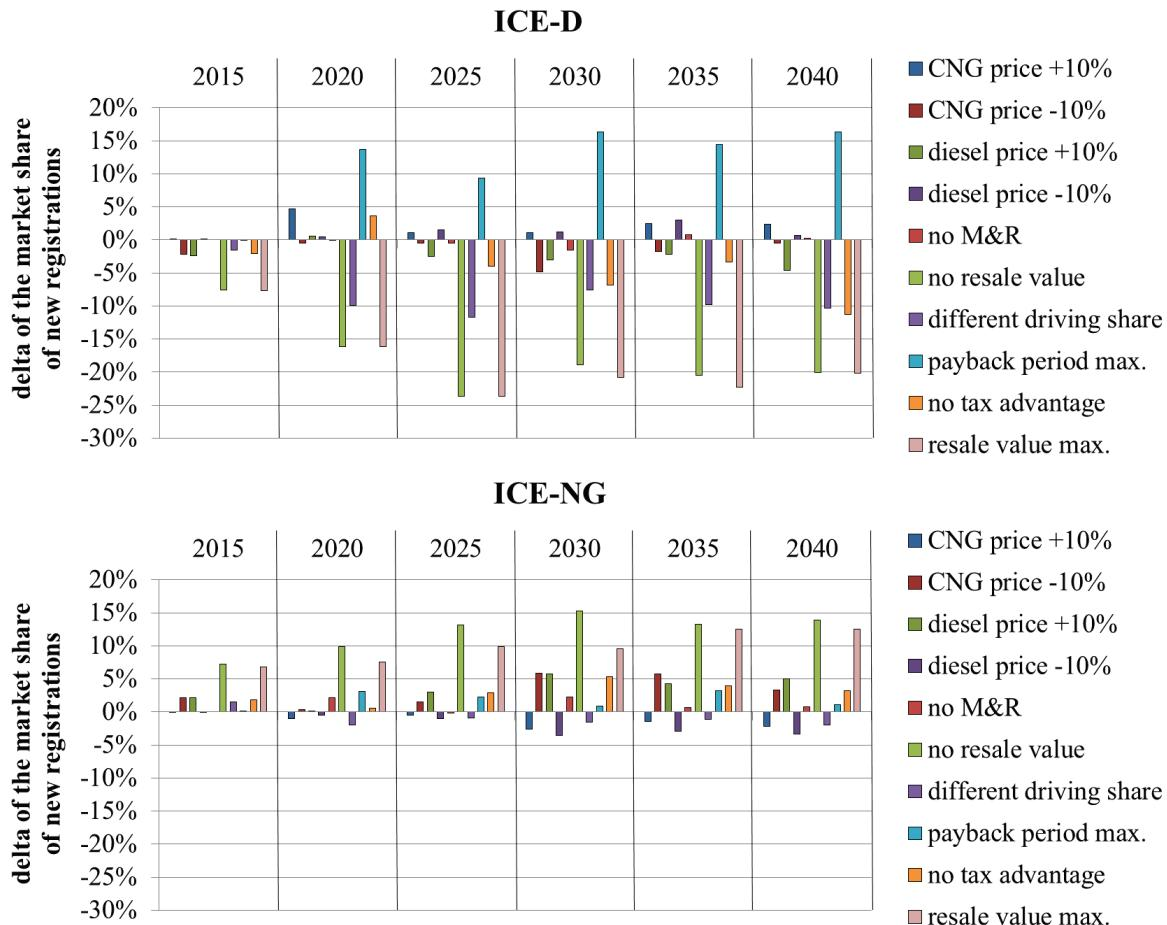
Figure 4: Results of the sensitivity analysis regarding the ICE-D and ICE-NG vehicle concepts
