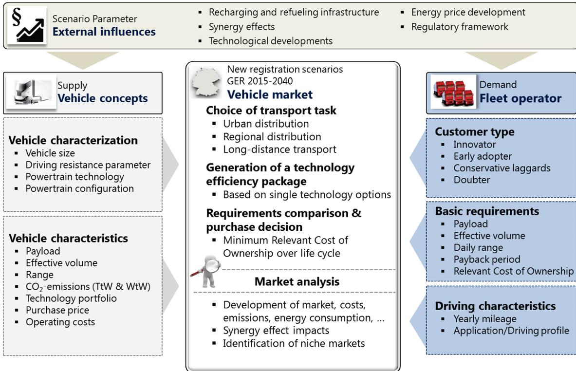
Figure 1: Approach of the road haulage vehicle technology market model
