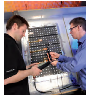
Fig. 2: Radiated sound power measured with sound intensity probe.
