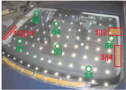
Fig. 1: Experimental setup of the active windshield with piezo-electric d_{31} -patches, electrodynamic shaker, accelerometers and laser-scanning grid (reflecting points).
