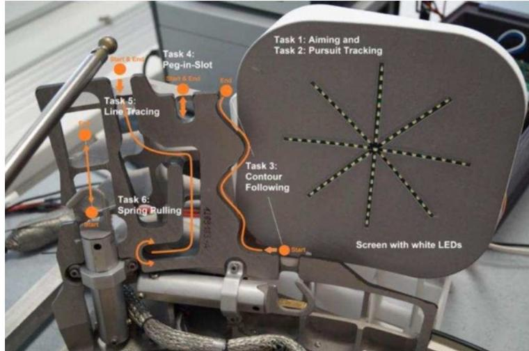
Figure 3: Task board for evaluating the performance of the telerobotics system
