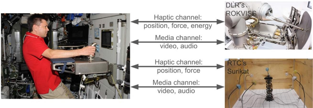
Figure 2. Telepresence data streams
