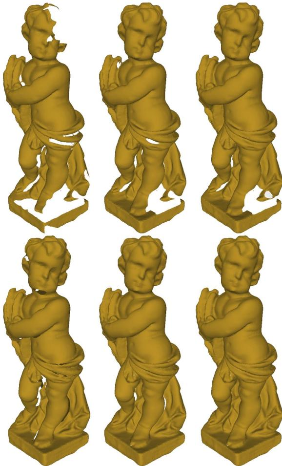
Fig. 3. The object coverage of the triangle meshes of the putto statue after 5, 15 and 30 scans (from left to right) are shown for *S/IG* (top) and *BH/IG* (bottom). *BH/IG* completes the mesh a lot better and contains less holes in each case.
