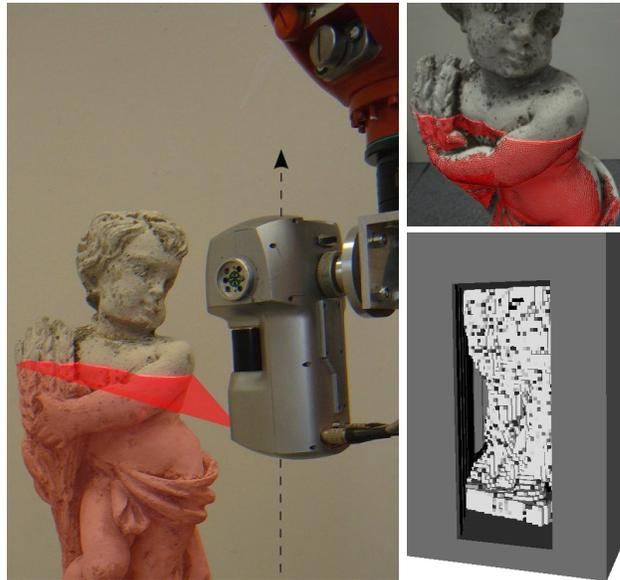
Fig. 1. *Left:* The robot is moved along a continuous scan path while the statue is scanned with the attached laser stripe profiler. *Upper Right:* A triangle mesh is reconstructed in a real-time stream during the sensor movement. *Lower Right:* The initially unknown space (gray) is updated based on sensor data of the current scan.
