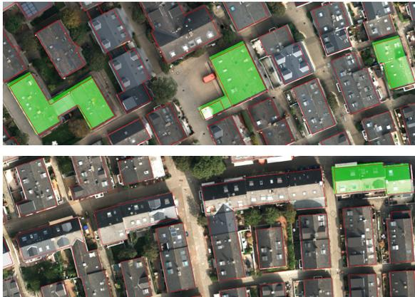
Figure 5. Comparison of the building outlines without roof overhangs (transparent green) and the cadastral map (red)
