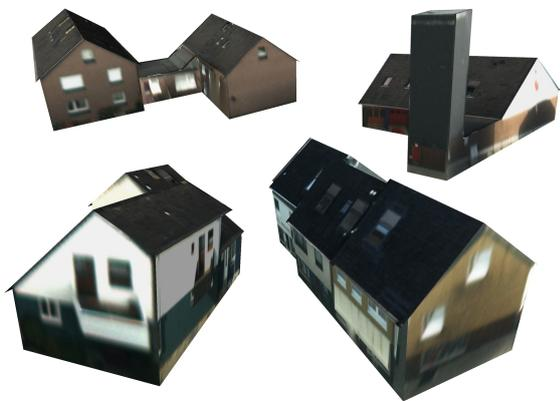
Figure 6. Textured buildings with discontinuities, roof overhangs
