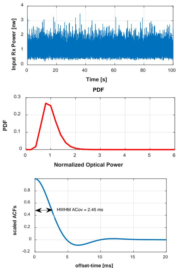
**Figure 4.** Generated Power Vector 1 with Power Scintillation Index of 0.1. Top figure shows normalized power samples w.r.t time, middle figure shows the pdf (lognormal) of the power and the last figure shows the auto covariance.
