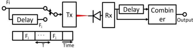
**Figure 3.** Block diagram showing delayed frame retransmission.  $F_i$  frame is transmitted once and retransmitted after a delay of  $T$  time.
