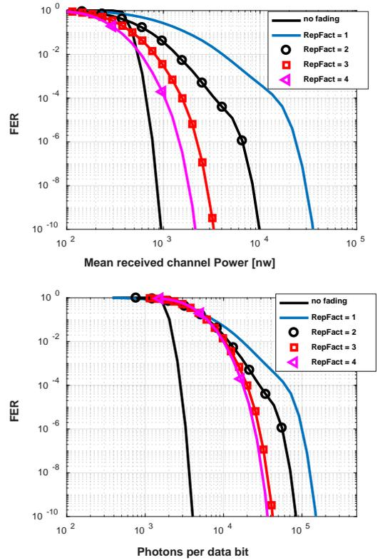
**Figure 8.** Performance in terms of mean received channel power (top) and photons per data bit (bottom), of DFR with MRC for the channel with  $\text{PSI} = 1$ ,  $\rho = 2$ .
