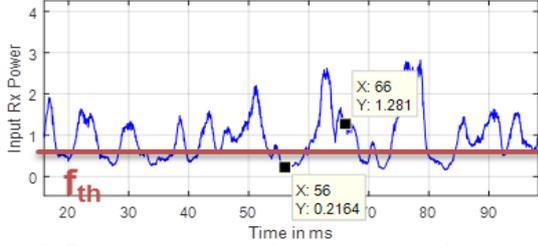
**Figure 2.** Excerpt of an example power vector showing fading threshold ( $f_{th}$ ) and fading/non-fading instances.
