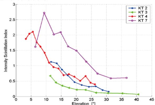
**Figure 1.** Intensity scintillation index derived from images of the “Profiler” camera vs elevation plot for different Trial #2, 3, 4 & 7 from KIDDO Downlink [1].
