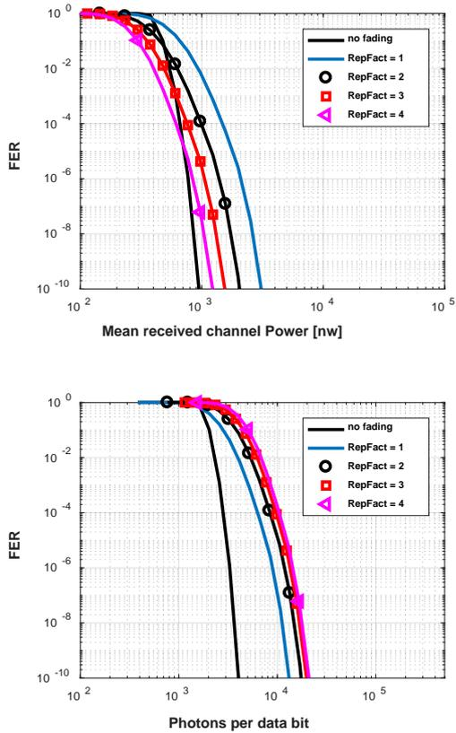
**Figure 5.** Performance in terms of mean received channel power (top) and photons per data bit (bottom), of DFR with MRC for the channel with  $\text{PSI} = 0.1$ , and  $\rho = 0.5$ .
