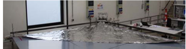
Figure 13. Fully deployed ADEO demonstrator after 2nd functionality test
