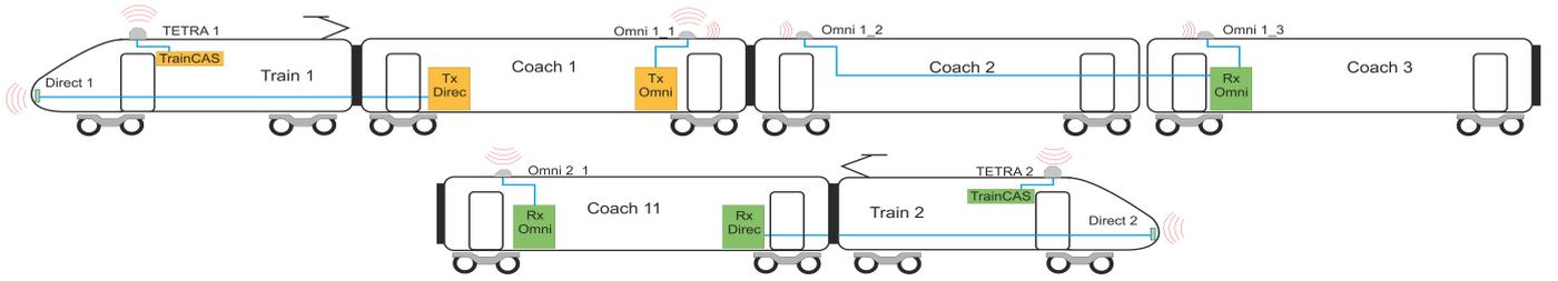
Fig. 3: Antenna setup for Train 1 (top) and Train 2 (bottom).
