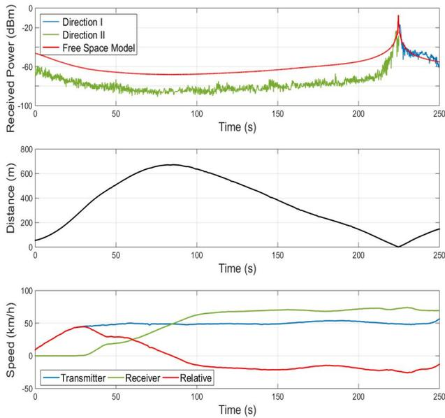
Fig. 4: Low speed overtaking maneuver in rural environment.
