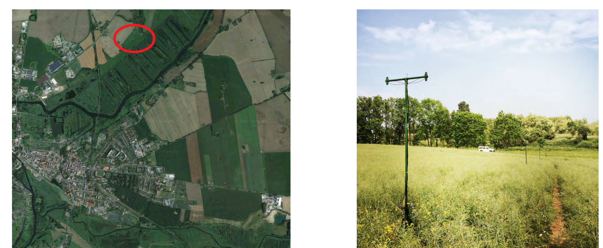
Figure 3: Left: Satellite image of the test site near Demmin, Germany. Right: Image of the wireless sensor network transect with increasing distance to the branch of the Peene river. The detected wavelengths of the multichannel sensors during the experiment were 665, 705, 740 and 865 nanometres for calculating a Normalized Difference Vegetation Index (NDVI) for canola.
