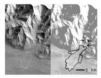
Figure 3. A landslide with a fan in Orbit 471.
