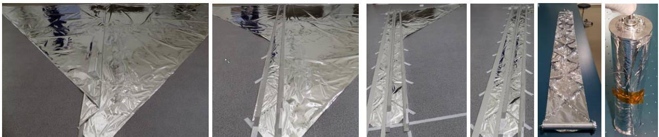
Fig. 8. Packaging of the Membrane folded parallel to the height and coiled onto the spool
