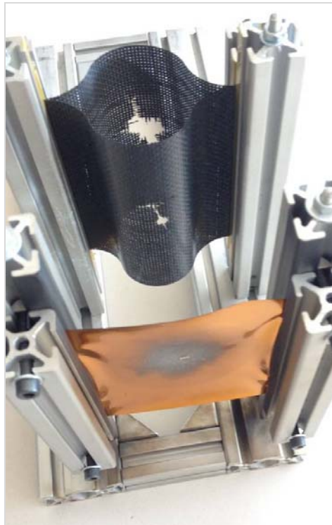
Fig. 17. Boom sample after impact
