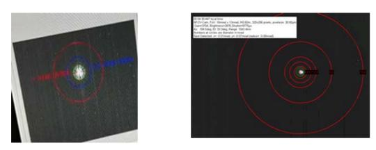
Fig 7. Tracking camera images of TOGS (left) and OGS-OP (right) after link acquisition and engagement of closed optical tracking loops. (Image source: DLR)
