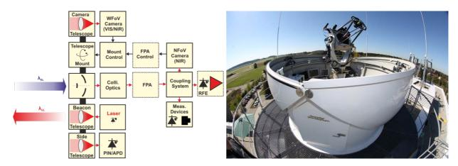
**Fig 5.** Left: generic functional block diagram of OGS-OP; Right: Image of open dome with 40 cm Cassegrain telescope (Image Source: DLR).
