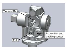
Fig 1. Scheme of the transmitter and coarse tracking sensor positions
