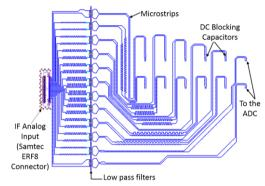
Fig. 2 Analog part for Ka band (layer L10)
