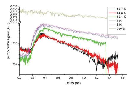
Fig. 4. Pump probe signals vs. delay time for the Ge:Sb sample at 141 µm wavelength at different sample temperatures; the upper signal demonstrates variation of input power during one of the experiments.
