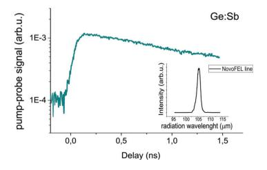
Fig. 2. Pump-probe signal vs. delay time for Ge:Sb sample at 105 µm wavelength, recorded at NovoFEL. Sample temperature: 5 K. Inset: NovoFEL emission line.
