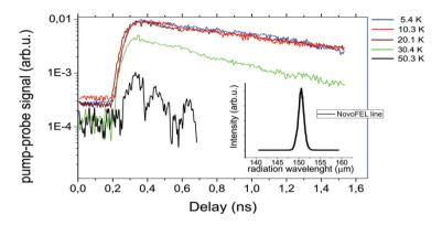
Fig. 3. Pump probe signal vs. delay time for Ge:Sb sample at 150 µm wavelength at different sample temperatures.
