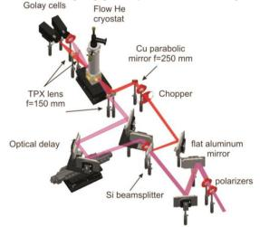
Fig. 1. Schematic presentation of single-color pump-probe setup at NovoFEL facility. Red line: pump beam, purple line: probe beam.
