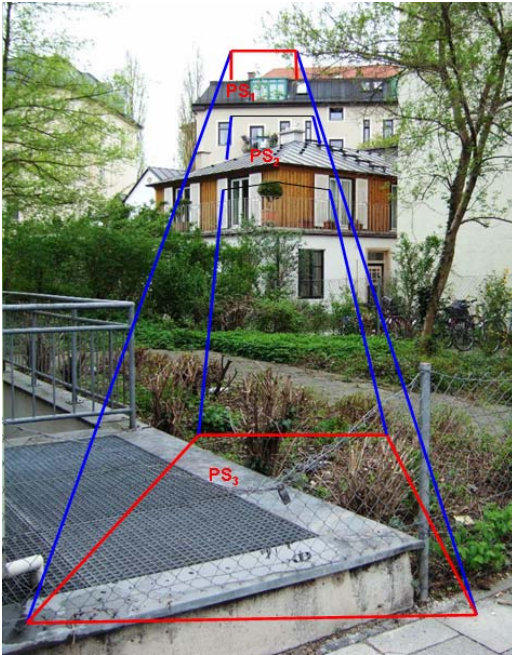
Figure 2: The 3D resolution cell is the volume inside the blue lines which run along cross slant range height. The red rectangle on ground is about 4 m x 30 m for the ERS sensor.
