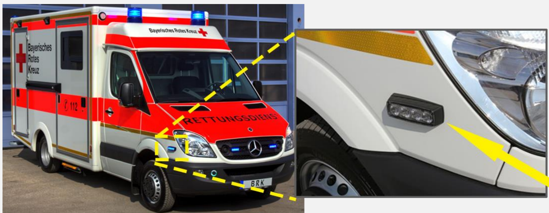
Fig. 1: Ambulance vehicle of BRK with additional beacon next to the headlights (left), additional beacon in close-up view (right)
