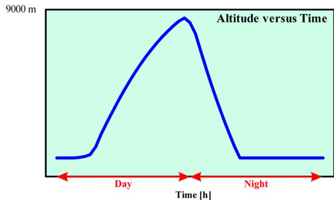
In order to obtain the smallest aircraft size (only 72 meters) the aircraft stores excess daytime energy in batteries and potential energy.
