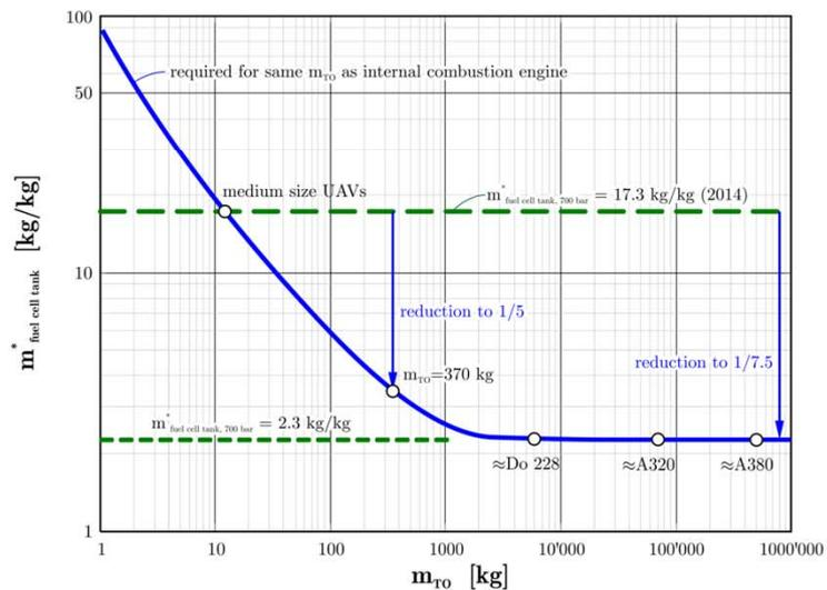
If we play the same game with a H<sub>2</sub> powered fuel cell system we can look at the pressurized hydrogen tank. These tanks are very heavy and technology is working towards lower mass.
