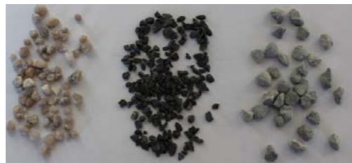
Figure 7 Selected natural stones (left: quartzite; middle: basalt; right: diabas)
