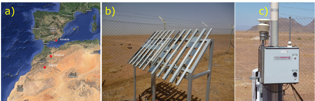
FIGURE 1. (a) Location of outdoor exposure sites in Morocco and Spain at the Plataforma Solar de Almería (PSA); (b) Outdoor exposure rack with reflectors in Zagora; (c) EDM164 particle counter from Grimm that was used on both sites to measure the particle concentration (location in this picture: Zagora).
