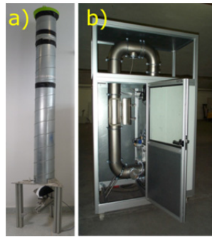
FIGURE 2. Artificial erosion setups in the laboratory. (a) Soil pipe, like proposed in DIN 52348 [20] and (b) closed loop SSC.
