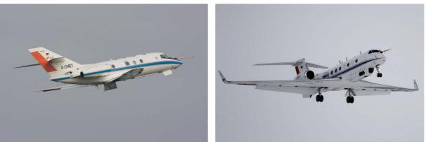
**Fig. 1.** Photographs of the airborne platforms carrying the DLR lidar systems. (a): DLR's Falcon 20 (D-CMET); (b): HALO, the German High Altitude Long Range research aircraft (D-ADLR). Here, the bellypod which can e.g. accommodate a radar antenna and an optical window aperture simultaneously is mounted below the aircraft's fuselage.
