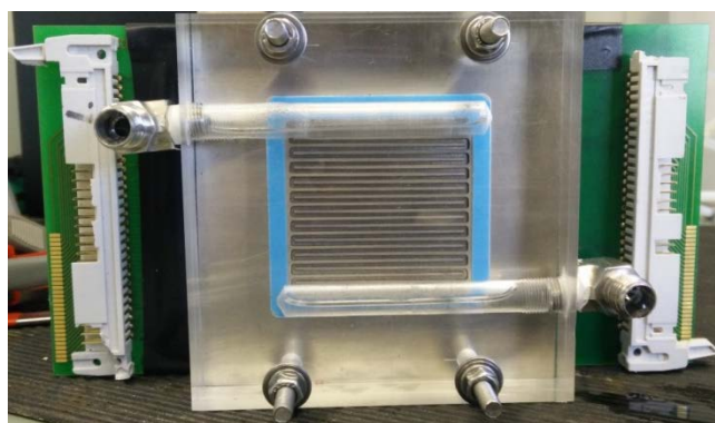
Figure 2. Successful integration of segmented PCB in PEMWE test cell with optical access
