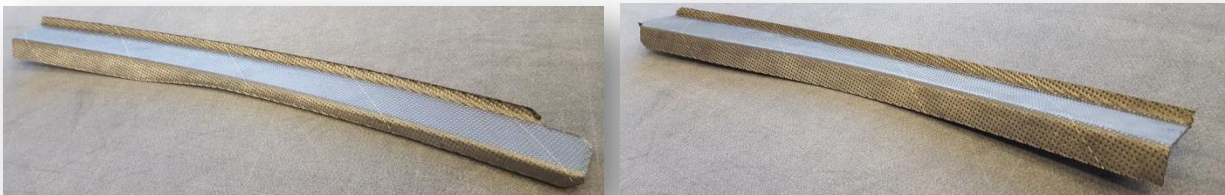
Figure 5: Net-shape preforms (left: upper C73 frame; right: lower C73 frame)
