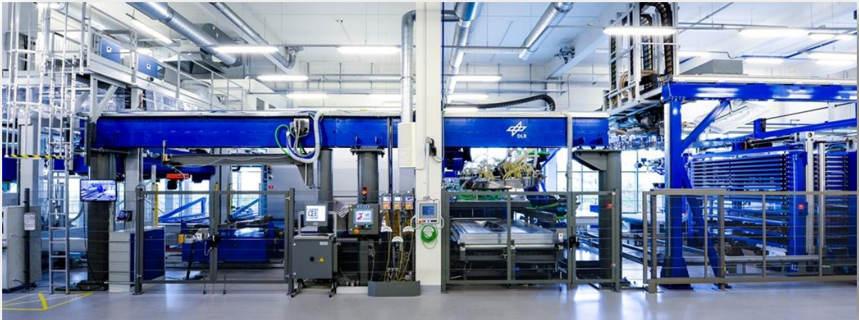
Figure 4: EVo facility – fully automated RTM production line
