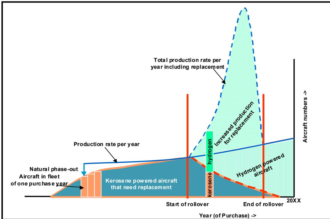
**Figure 77: Accelerated kerosene to hydrogen fleet rollover**
