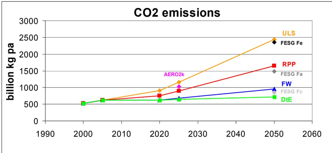
Figure 39: Comparison of CO2 emissions with AERO2K and FESG
