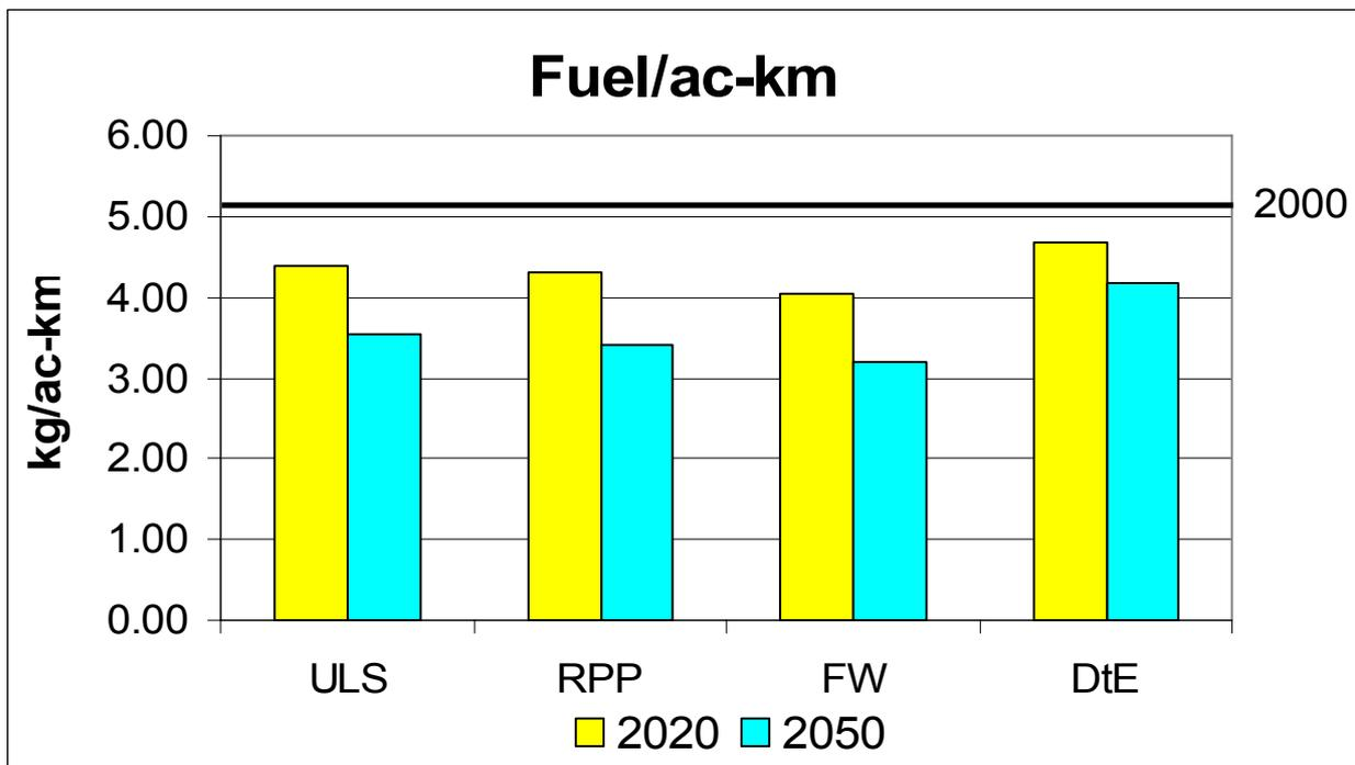
Figure 35: Specific fuel consumption (Fuel/ac-km)
