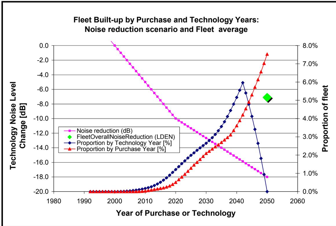
Figure 53: Fleet built-up by purchase and technology years: noise reduction and fleet average (typical for an expanding fleet)
