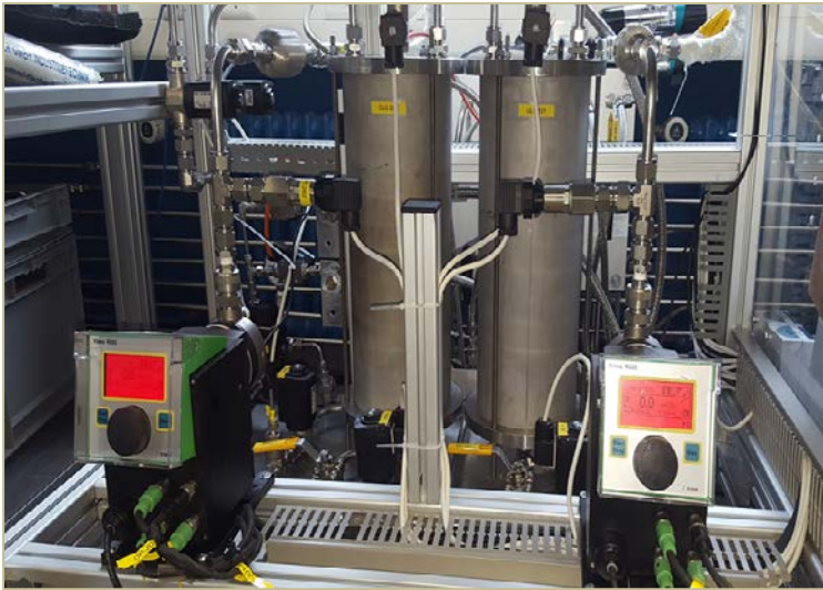
Figure 3 : Two Water pumps and Hydrogen H_2 - Oxygen O_2 storage
