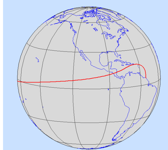
Figure 6: SpaceLiner 7 Orbiter final phase of reentry ground track
