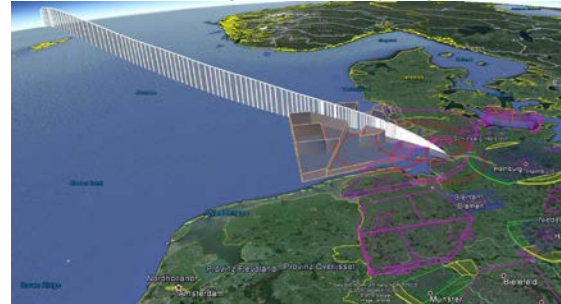
Figure 26: SpaceLiner final approach trajectory for destination in northern Germany; showing also danger areas, restricted areas and temporary restricted areas within German airspace 1
