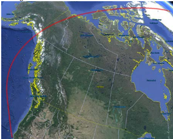
Figure 24: Simulated SpaceLiner 7-100 descent ground track nominal mission Europe to California
