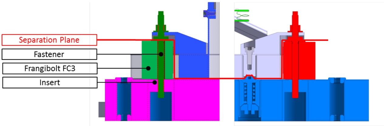
Figure 3 Overview of the separation mechanism between the Cradle and the Support System
