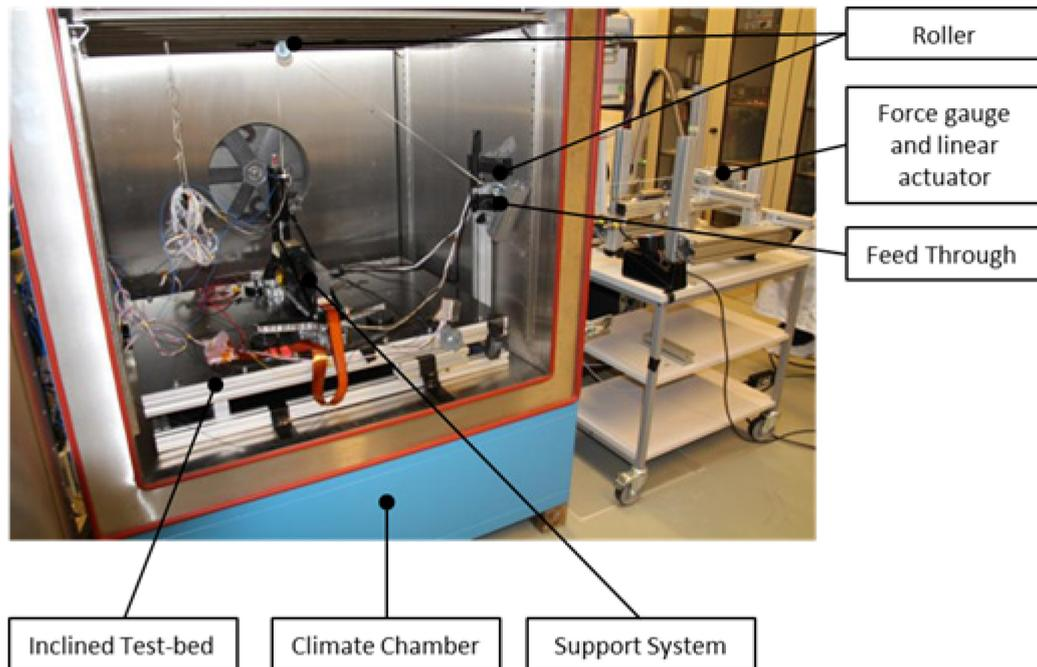
Figure 6 Overview of the test setup for the Cradle to Support System Separation Test
