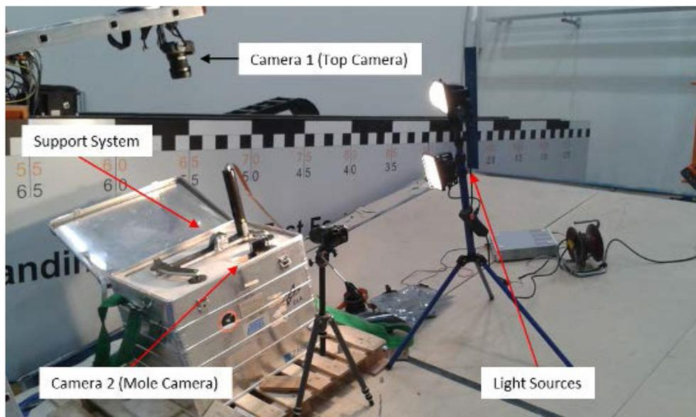
Figure 7 Overview of the test setup for the Feet Sliding Resistance test
