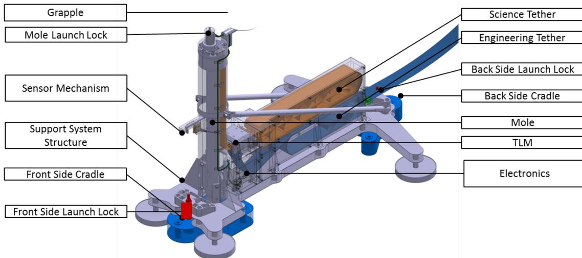
Figure 2 Overview of the sub-systems of the HP<sup>3</sup> Support System
