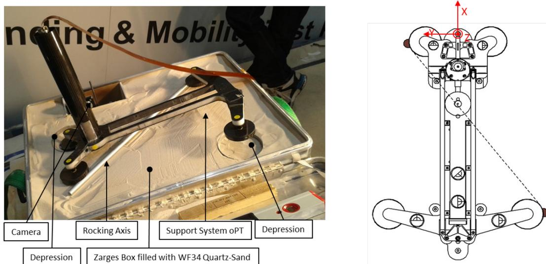
Figure 8 Left: Overview of the test setup of the Rocking Test. Right: Schematic topview with rocking axis and coordinate system
