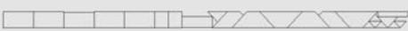
Fig. 3: Nesting for a skin part preform out of sliced UD layers, material utilization degree ≈ 95%.
