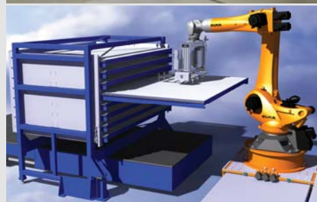
Fig. 6: Drawer storage with cut-pieces on its way to a robot cell (above) and picking out of drawer storage (below)
