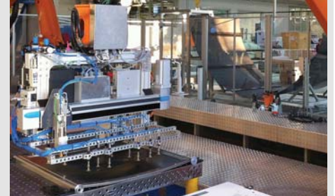
Fig. 7: Robotic pick and place end-effector.
