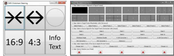
Fig. 3. Screenshots of the simplified (left) and comprehensive (right) video signal routing app.
