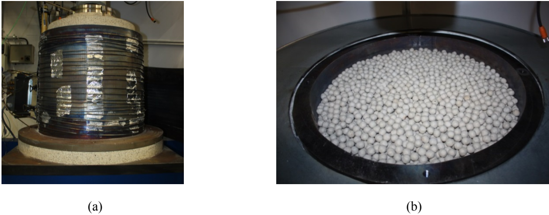
FIGURE 1. a) Cylindrical pressure cell; b) Pressure cell containing the packed bed
