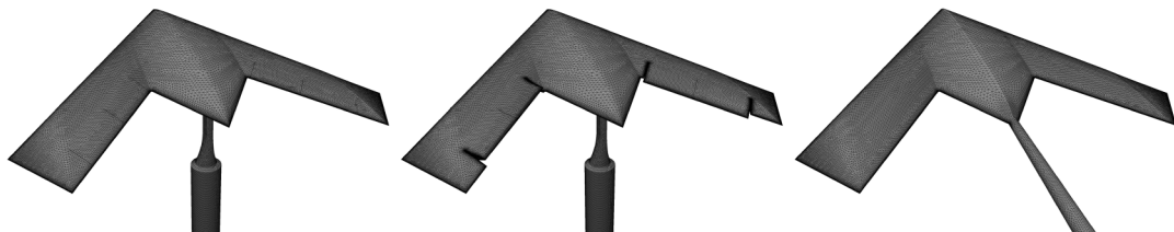
Fig. 9 Grid 2 surface triangulations for DLR-F19 with CS0 and CS20, and DLR-F17 with aft sting. Left to right: G2.00, G2.20, and G2a.
