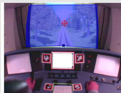
Figure 2. Eye tracking with D-Lab 3.0. Defined AOI (Areas of Interest) top down: track, display, timetable.
