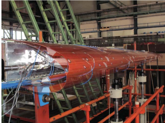
Fig. 3: Large scale ground test of the enhanced adaptive droop nose.
