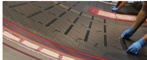
Fig. 10: Lay-up of SHM arrays on uncured skin
