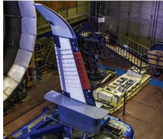
Fig. 4: Smart leading edge integrated in the outboard wing demonstrator.
