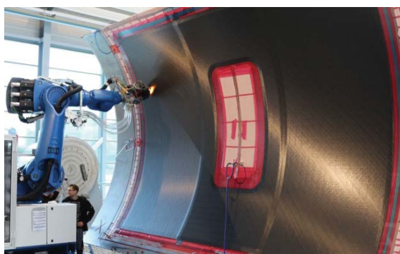
Fig. 9: Skin lay-up by automated fibre placement
