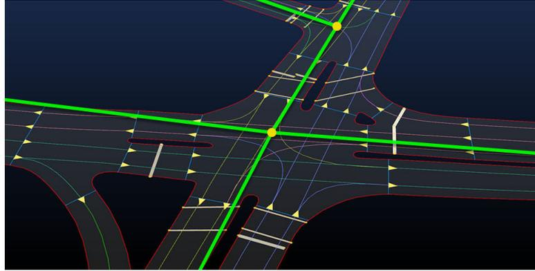
**Fig. 2.11** – Comparison of standard map and next generation road map model from Nokia HERE [57]. The road geometry in the standard map is defined by polylines (green). The HD map format underneath uses more complex geometrical primitives for a precise representation of the geometry at the lane-level than the standard map.
