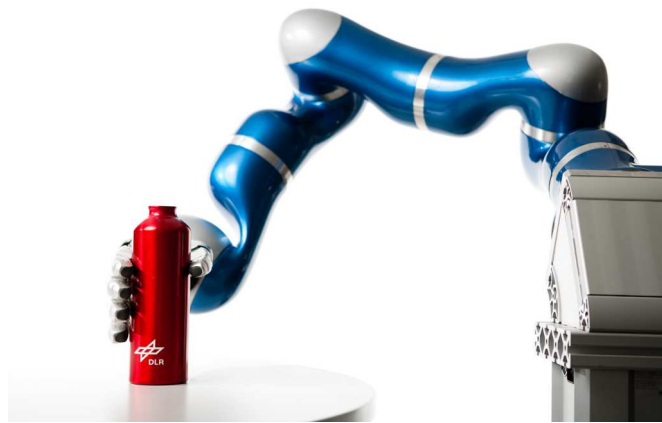
Fig. 1. The DLR Light-Weight-Robot - a sensitive torque controlled robot for safe human robot collaboration
