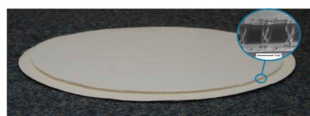
E-bypass separator (top); inset: SEM image of cross section (top); KOH flow concept in system using e-bypass separator (bottom). VITO
