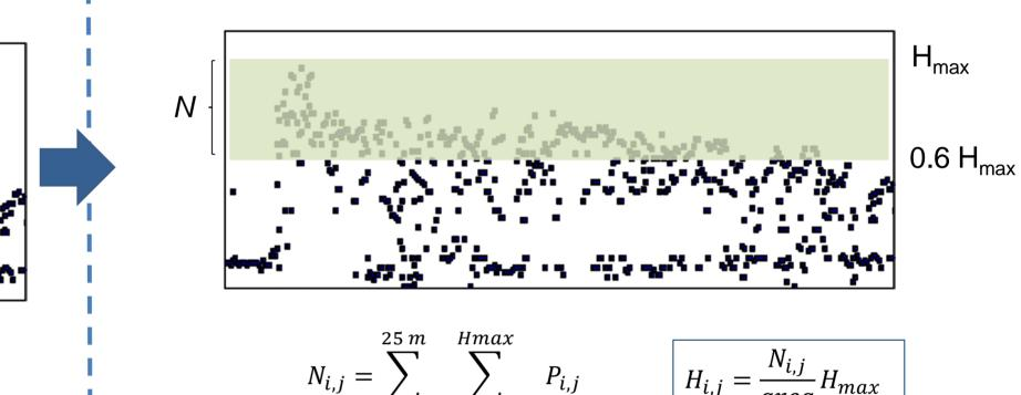
Where  $P_{i,i}$  is a binary matrix with non-zero elements at the position of every *peak* and  $\sum_{i,j}^{25 m}$  denotes the window of 25 by 25 meters around the pixel i,j.
