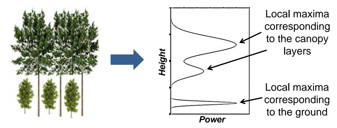
Correspondence between canopy layers and 3D reflectivity from TomoSAR measurements
