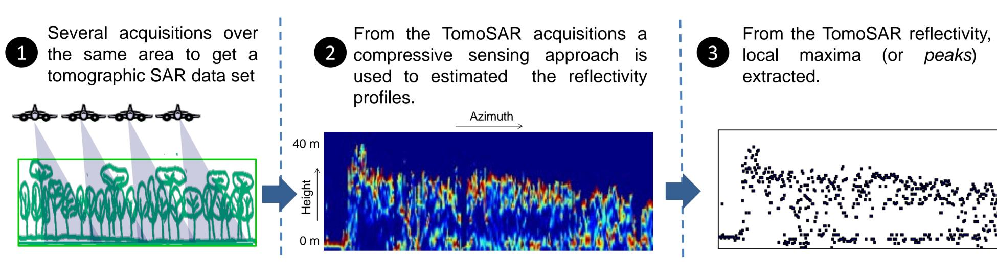
From the distribution of local maxima, two forest From the TomoSAR reflectivity, the structure indicators, both in vertical and horizontal local maxima (or *peaks*) are directions, are estimated.
