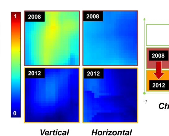
After a strong logging in a density of trees decreases and, as a consequence, the horizontal descriptor higher (low density) while the vertical remains stable because the variability in the vertical direction is not changing.
