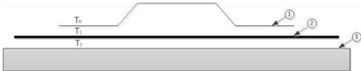
Figure 6 Trial setup with Omega stringer (1), prepreg laminate (2), tool (3) and the positions of the temperature measurements (on the left)
