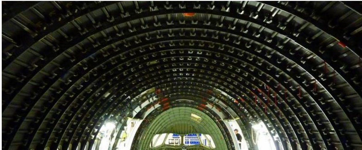
Figure 1 Stringer and Frame Stiffened Shell Structure of an A350 [5]
