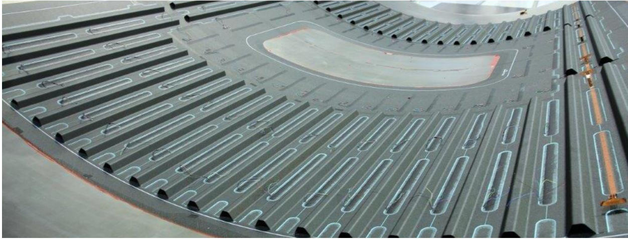
Figure 11 Full Scale Pre-Bonding Tests A350 XWB shell - skin layer setup without ramps (constant thickness)
