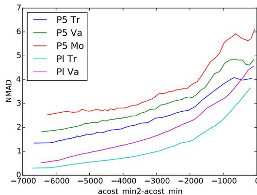
Figure 6: Dependence of height error on difference of first and second aggregated cost minima  $A_{mmn}$ .
