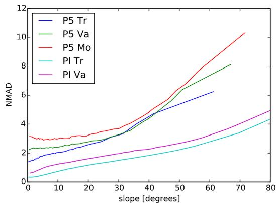
Figure 4: Dependence of height error on slope for Cartosat-1 (P5) and Pleiades (PI) DSMs.
