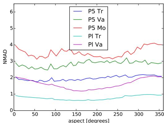
Figure 5: Dependence of height error on aspect.
