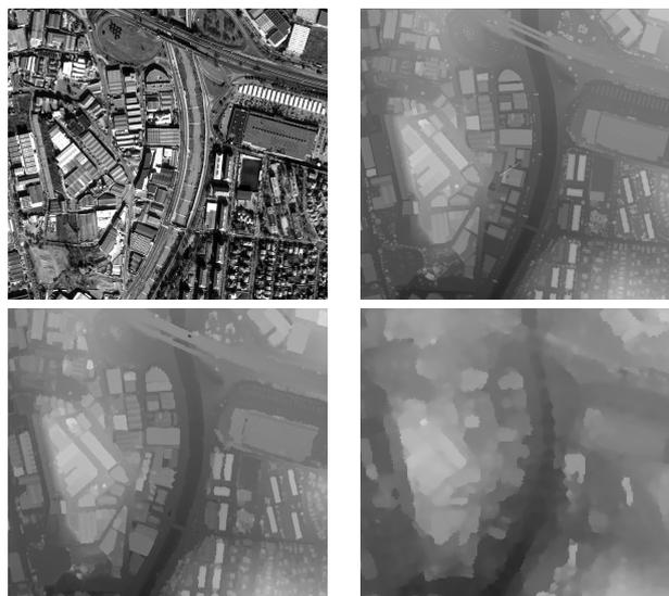
Figure 3: Detail of MGM8 results on the Terrassa area. Top row: Pleiades ortho image, LIDAR reference. Bottom Row: Pleiades DSM, Cartosat-1 DSM.
