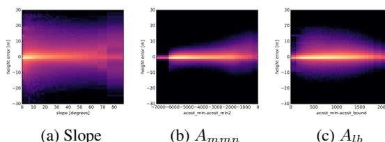
Figure 8: Height error vs. confidence variable joint histograms for the Pleiades Terrassa triplet. Color is proportional to the logarithm of density of each joint histogram bin.
