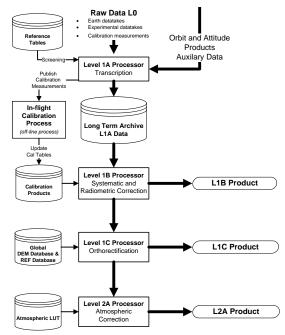
Figure 4 Processing chain and product generation
