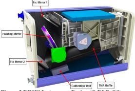
Figure 2 DESIS Instrument Design (© DLR-OS)
