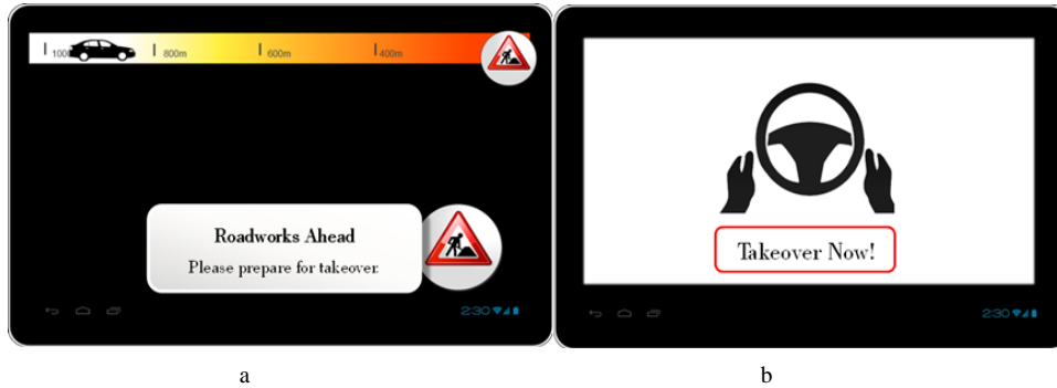
Figure 2: Early information about a pending takeover request due to roadworks (a) and the takeover request on the tablet-pc of the driver (b).
