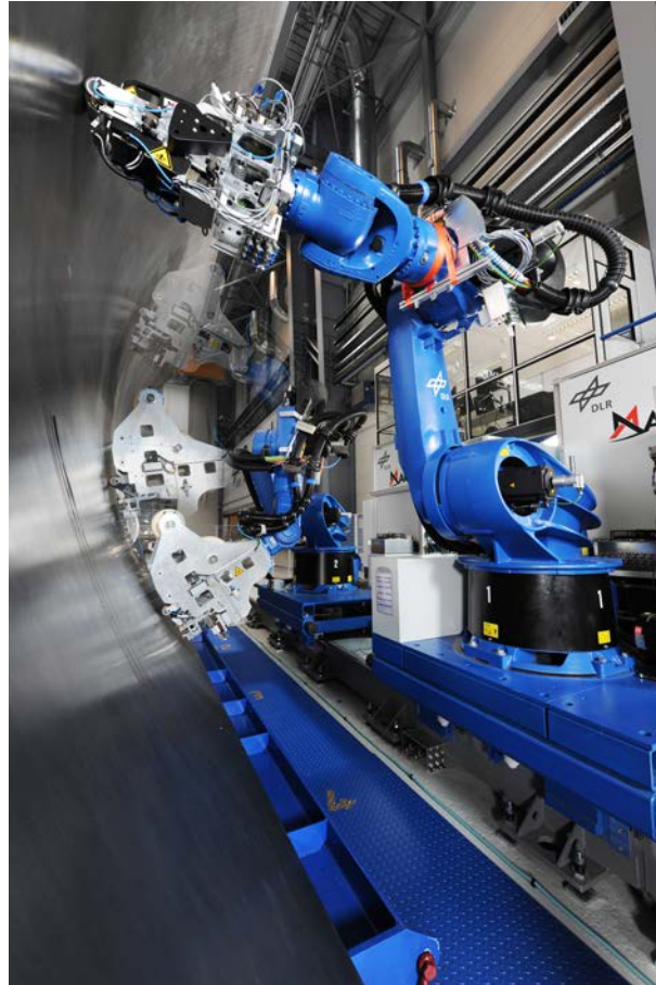
Figure 3: GroFi - realizing a combined usage of fiber placement and tape laying technology
