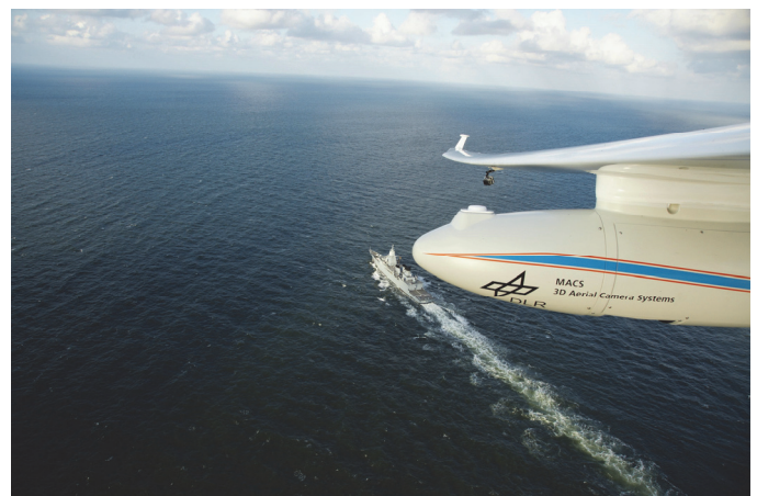
Fig. 1. Preliminary version of MACS-Mar mounted in a underwing pod of a Stemme S10 VTX motorglider
