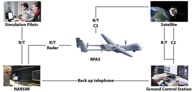
Figure 4 RPAS simulation architecture
